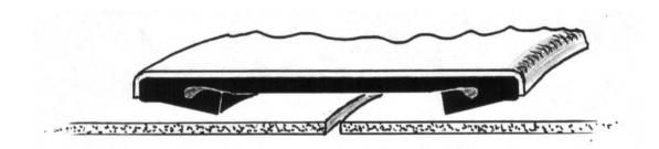
The gasket itself has sealing lips which press against the pipe surface and forms lip seals. The lip seals are designed to resist the internal pressure in the pipes. As the pressure increases, the coupling is designed to seal more tightly against the pipe surface.
