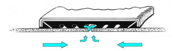
Under pressure, or external load, as the pipes try to pull apart, the anchor rings rotate, which pushes the outer edges of the casing upwards. Under the ensuing beam effect the central cross section of the casing bows inwards which further compresses the rubber to form a yet tighter seal against the pipe.
