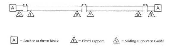
Intermediate anchors should be designed to withstand the forces and movements transferred and imposed upon them by each of the pipe sections to which they are attached, taking into account such forces as friction, wind load, self weight, and changes in fluid momentum.
