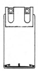
Teekay **Bracketed** Pipe Couplings can be provided with brackets of various designs welded to the coupling casing which can then be bolted to any convenient support.
