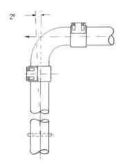
Teekay **Axiflex** Couplings can accept thermal expansion or contraction of the pipeline by axial movement through the coupling or by the angulation of two couplings. In either case the pipeline should be adequately restrained.
