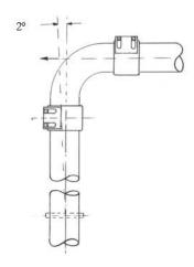
Teekay **Axilock** Pipe Couplings should always be installed in accordance with good piping practice, conforming to the relevant industry standards. For example:
