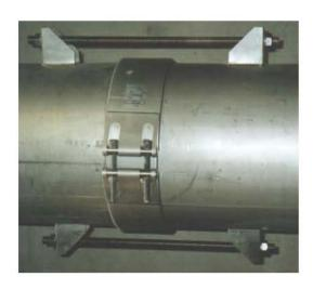
For above ground applications where there is a possibility that the coupling may move along the pipe due to excessive vibration, expansion and contraction etc. the Teekay **Axiflex** Pipe Coupling can be supplied with a central register. The central register is a circumferential ridge integral to the gasket and serves to locate the coupling on the pipeline, thereby preventing its movement. (This should be specifically requested at time of order.)
