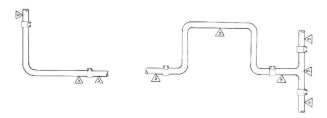
Standard Teekay **Axiflex** Pipe Couplings are not designed to accept end load pressures. As a result, pipes must generally be anchored against internal pressure at changes in direction, branches, valves and at pipe ends. For example:
