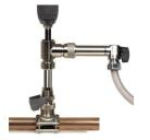
When the drill housing is removed halfway, the non-return valve closes stopping the flow of water in the hose.
